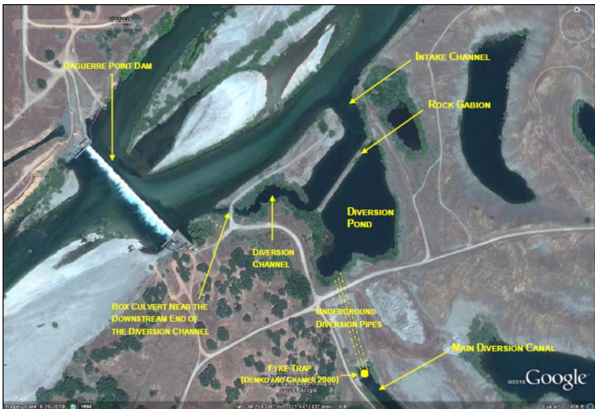
15 16 Figure 5-6. Diversion headworks area for the South Yuba/Brophy Diversion Canal and 17 Facilities.
