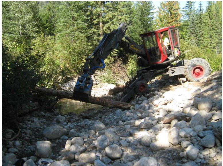
Figure 5. “Spyder” excavator (Source: ArcRidge LTD Environmentally Responsible Forest Services 2011).
